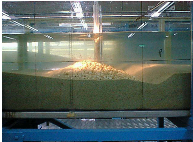
Figure 5. Formation of riprap mound around bridge pier in a degrading bed (Flow from right to left)
