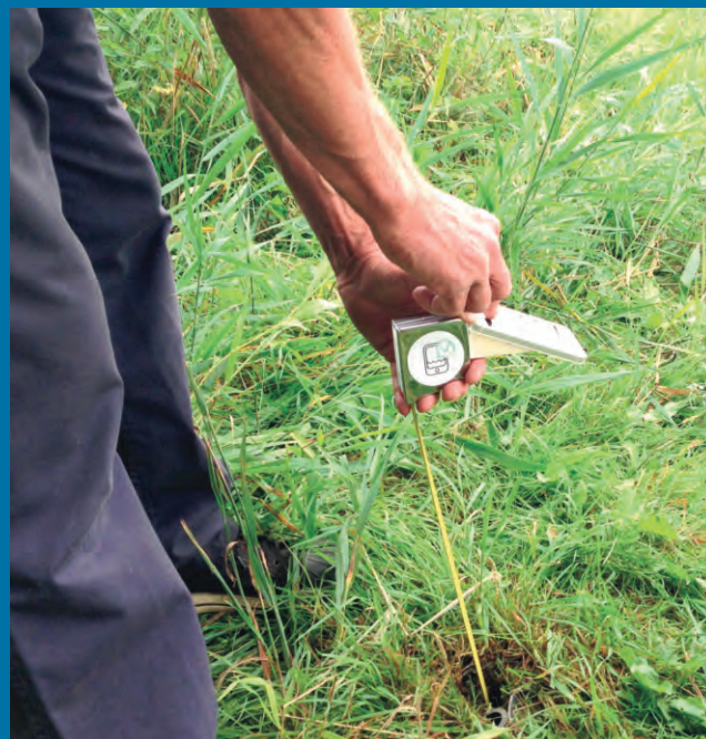
Figure 3. Mobile Tracker measuring a ground water level
