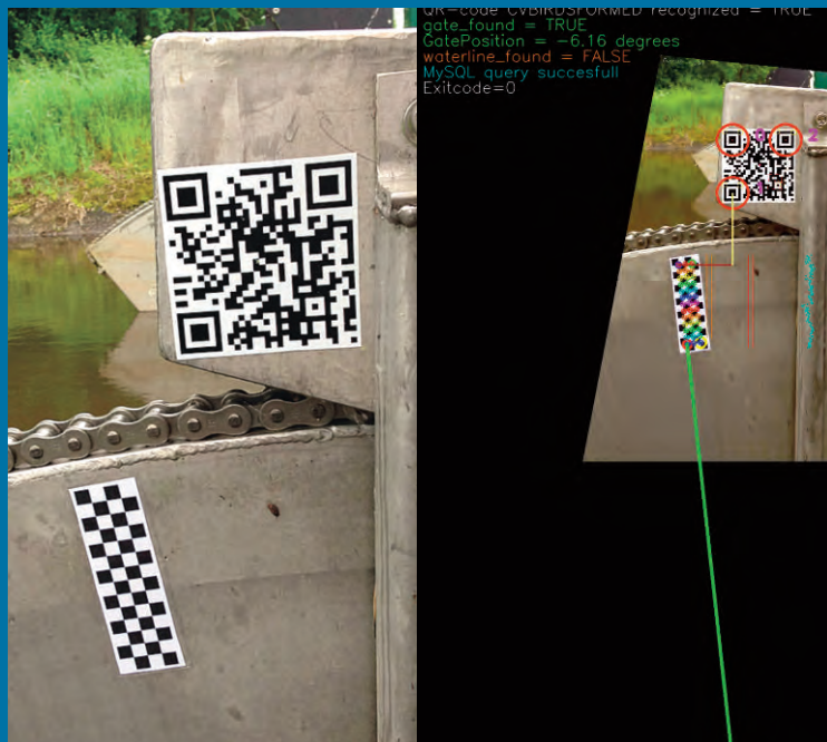
Figure 2. Mobile Tracker measuring a gate position (on the left is the original photo, on the right the manipulated photo with the perspective correction and how the angle resulting in the gate position is determined)
