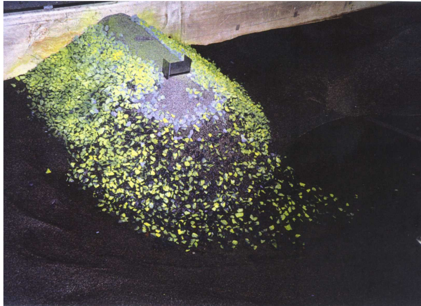
Fig. 2. Failure of riprap on an abutment in a laboratory experiment (Eve, 2000).
