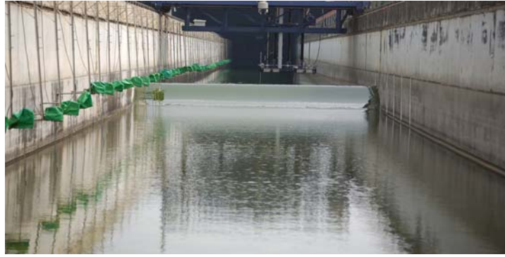
Figure 1 Laboratory image of a solitary-wave-type tsunami propagating toward a 1:60 sloping beach in the present supertank (offshore view).
