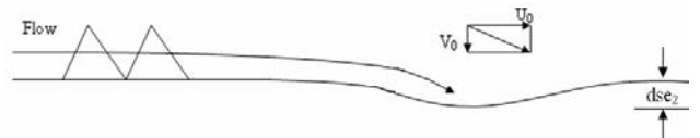
Figure 6. Sketch of the flatness and scour hole formed downstream of the tetrahedron frame layer
