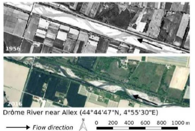
Figure 1: Examples of channelized gravel bed rivers located in the French Alpine region between 1956 and 2016, showing the development of vegetation on alternate bars (source: IGN) [5]
