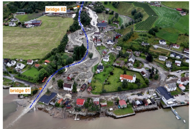
Figure 2. Aerial view of Utvik flood event from the fjord [4], with original river thalweg (blue line) and bridges.
