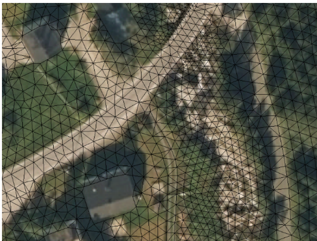
Figure 3. Example of the mesh (cell size is 2 m in the river channel and 3 m in the rest of the domain). Buildings are cropped out of the mesh.
