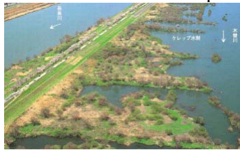
Fig. 1. Spur dikes and “Wando” in Kiso River
