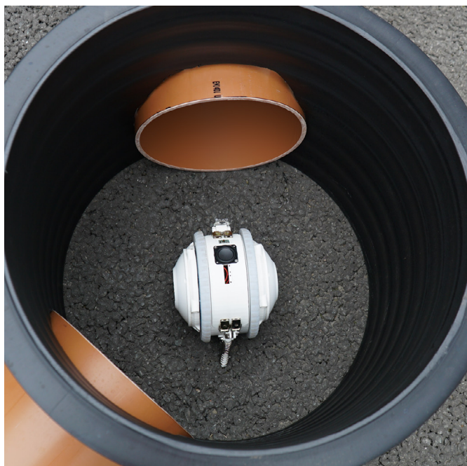
Figure 3 | Sprintbot first prototype testing in mock pipe network.
