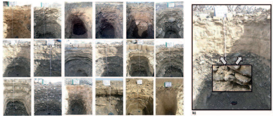
Figure 5. (a) Soil Pedons of the Al-Khoud dam bed, about thirty (30) years after the dam commission, (b) a typical soil profile illustrating the sedimentation in Al-Khoud reservoir and the deep percolation of fine particles into the original gravelly alluvium
