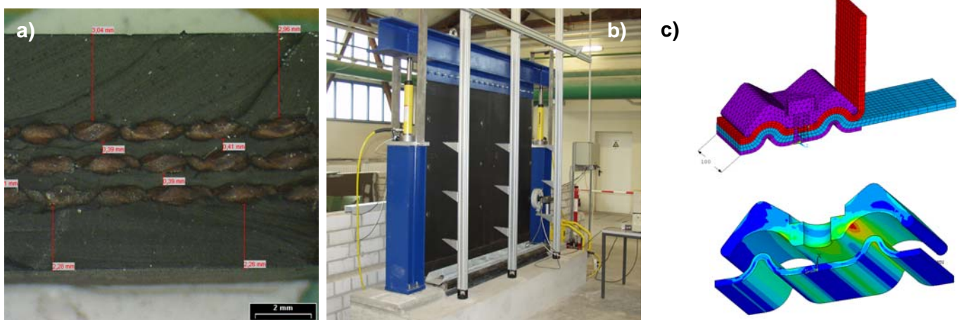
Figure 5: a) Micrograph of a three-layer, 12 mm thick tubular membrane b) Long-term behaviour test rig c) FE model and stresses in the steel rails
