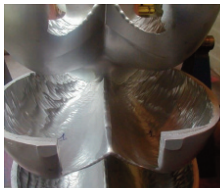
Figure 5. Abrasion on Pelton runner (source: EDF)
