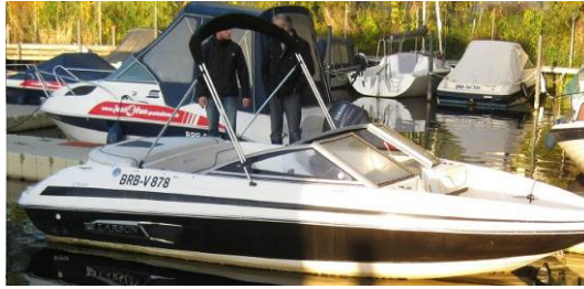
Figure 5 Boat type 4 – motor boat “Larson LX 850”, 4-stroke-inboard engine (petrol), power 99.3 kW
