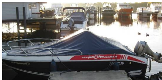
Figure 4 Boat type 3 – motor boat “Galia 475”, 4-stroke-outboard engine (petrol), power 5.9 kW
