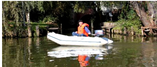
Figure 2 Boat type 1 – rubber dinghy “Typhoon 310 Aero”, 2-stroke-outboard engine (petrol), power 3.7 kW
