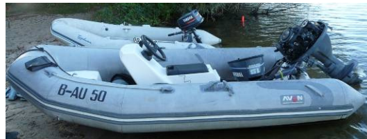
Figure 3 Boat type 2 – inflatable dinghy “Avon R340”, 4-stroke-outboard engine (petrol), power 11.0 kW
