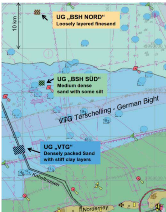
Fig. 2: Test-sites in the German Bight with a brief description of the sediments
