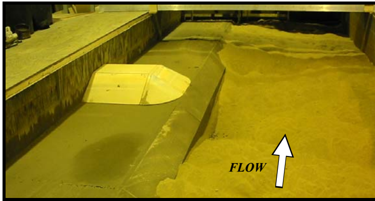
Figure 2. Scour in main channel near fixed floodplain and embankment (flume width is 4m)
