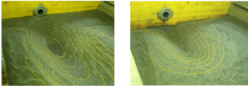
Figure 3: Scour hole for D = 10 cm and Q = 12.5 l/s; high tailwater h_{TW}/D = 1.1 (left), low tailwater h_{TW}/D = 0.2 (right)
