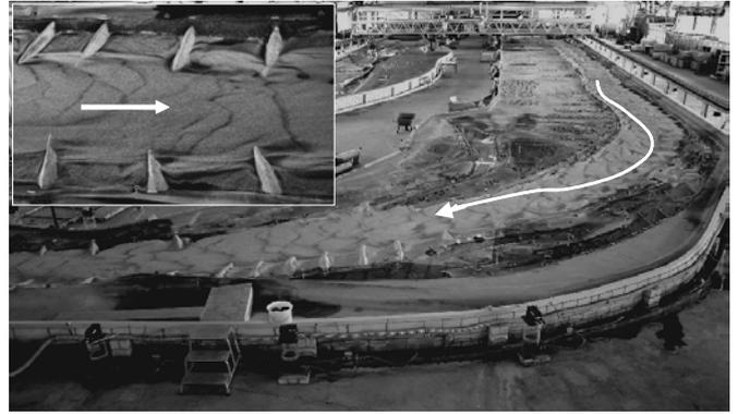
Figure 1. View of the model and detailed photograph of bed forms and training structures.
