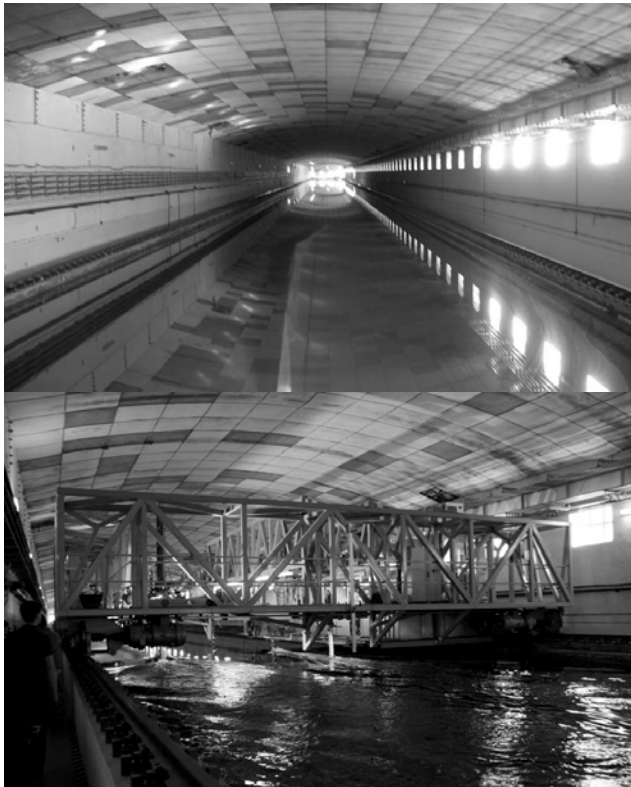
Figure 1: CEHIPAR Ship Canal Facility. The upper photograph shows the canal and the lower photograph the carriage on rails suspended over the canal.
