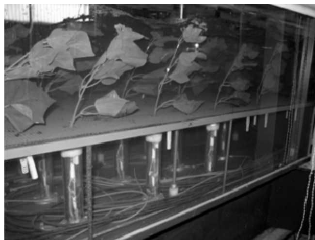
Figure 1: Setup of DFS test section and artificial poplars under flow action.
