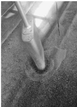
Figure 10. Photograph showing scour around round nosed pier
