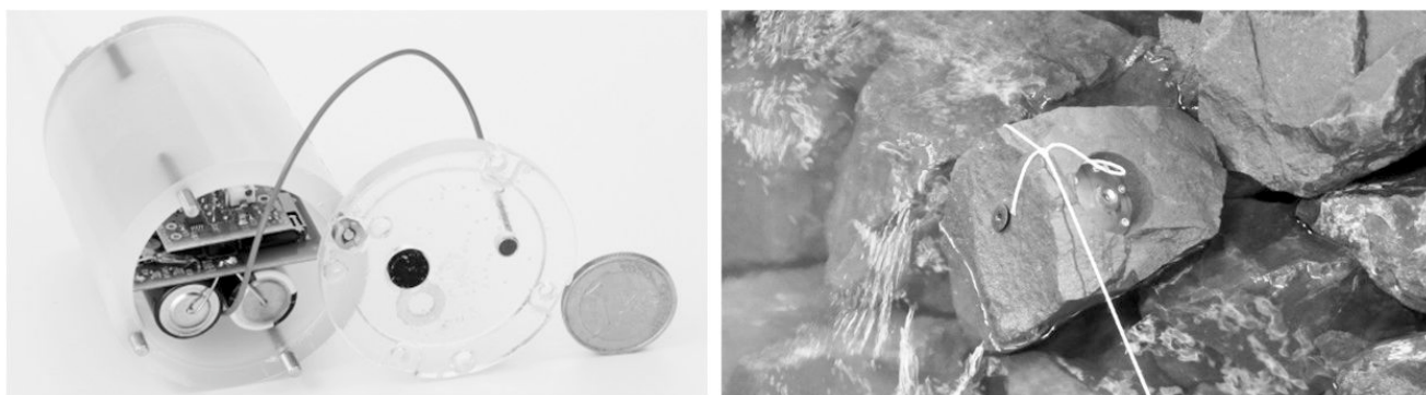
Figure 5. Example of armourstone equipped with sensor technology.
