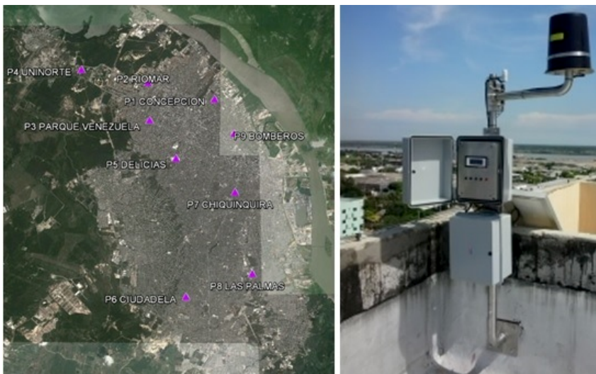
Figure 5. Location of rain gauges monitoring network (left) and rain gauge installed (right). Source: Authors.
