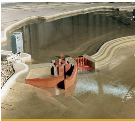
Figure 2. Physical model at HR Wallingford with Gibb design
