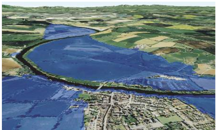
Figure 2. 3D visualisation of flooding (ISIS 2D)
