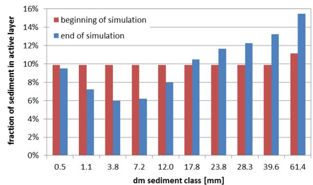
Figure 8: Simulated mean fraction of sediment classes for the active layer.
