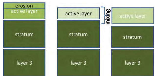
Figure 2: Erosion procedure for Hirano-Ribberink model in SISYPHE
