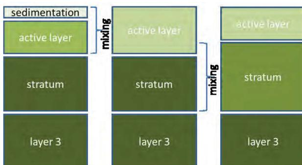
Figure 1: Sedimentation procedure for Hirano-Ribberink model in SISYPHE.
