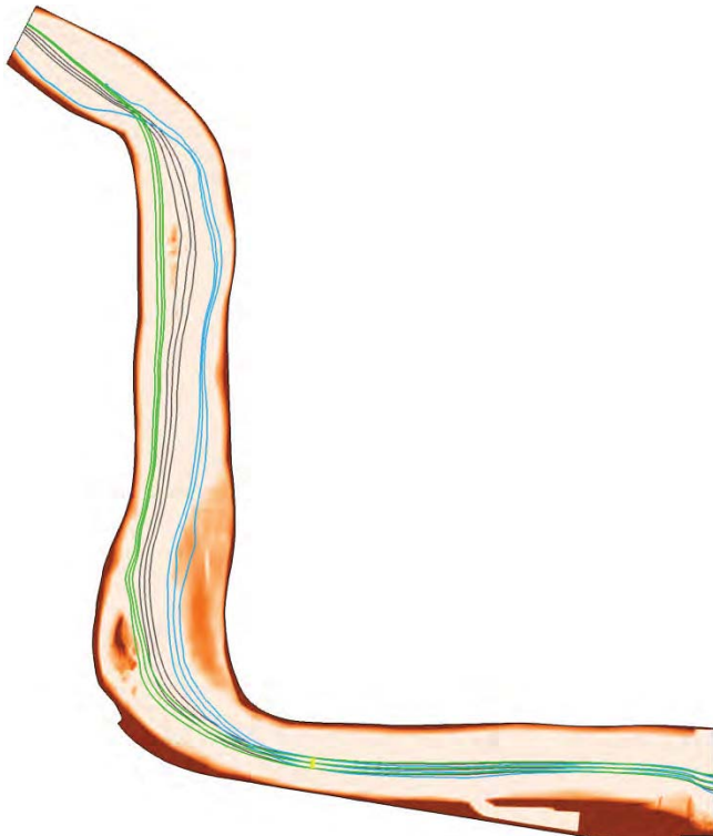
Figure 10: Streamlines nature-scale model, Nat_n10 Chézy scaled (grey: depth-averaged velocity, green: velocity at the free surface, blue: near-bottom velocity)
