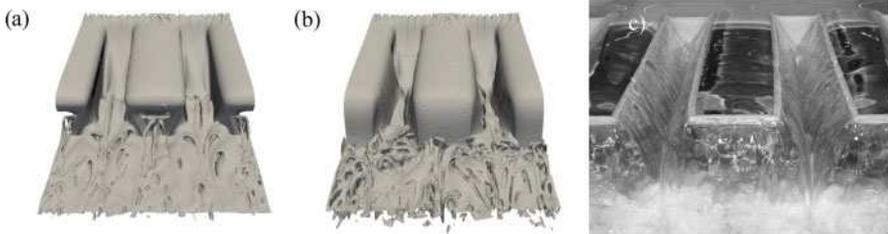
Figure 6. Numerical results for un aerated flow (a) and aerated flow (b) in comparison with physical experiment (c) for  $q = 0.04 \text{ m}^3/(\text{sm})$ .
