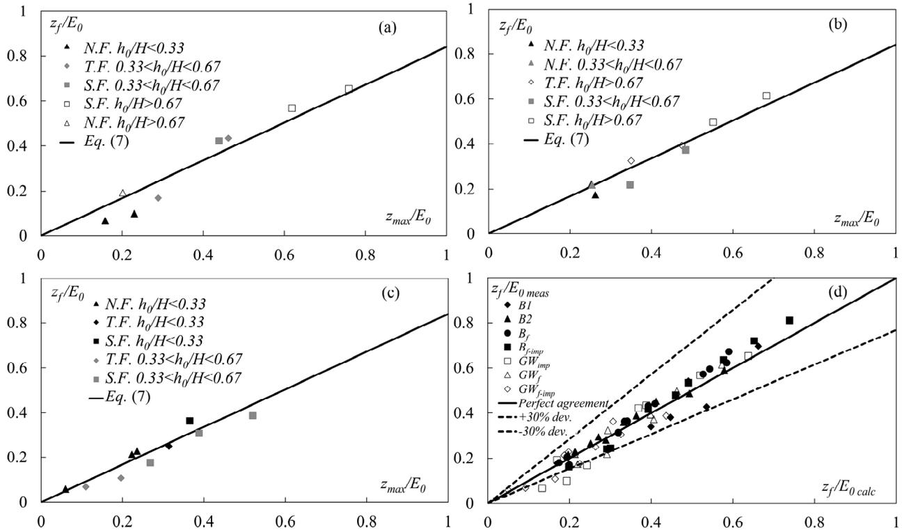
Figure 5.  $z_f/E_0$  versus  $z_{max}/E_0$  for different flow regimes (N.F.=Nappe Flow, T.F. Transition Flow, S.F.=Skimming Flow) and relative submergence and for stepped gabion weirs (a)  $GW_{imp}$ , (b)  $GW_f$ , (c)  $GW_{f-imp}$ . (d) Comparison between measured and calculated values of  $z_f/E_0$  using Eq. (6) (rock grade control structures) and Eq. (7) (stepped gabion weirs)
