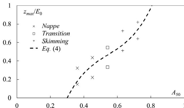
Figure 3. Non dimensional scour depth as function of  $A_{50}$  for different flow regimes and rock grade control structure  $B_{f-imp}$
