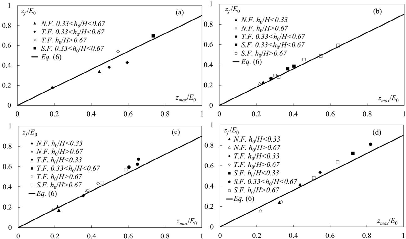
Figure 4.  $z_f/E_0$  versus  $z_{max}/E_0$  for different flow regimes (N.F.=Nappe Flow, T.F. Transition Flow, S.F.=Skimming Flow) and relative submergence and for rock grade control structure (a)  $B1$ , (b)  $B2$ , (c)  $B_f$  and (d)  $B_{f-imp}$
