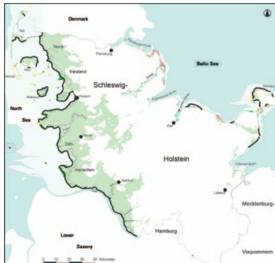
Fig. 1: Overview of Schleswig-Holstein with State dikes (black bold lines), regional dikes (brown lines), and coastal lowlands
