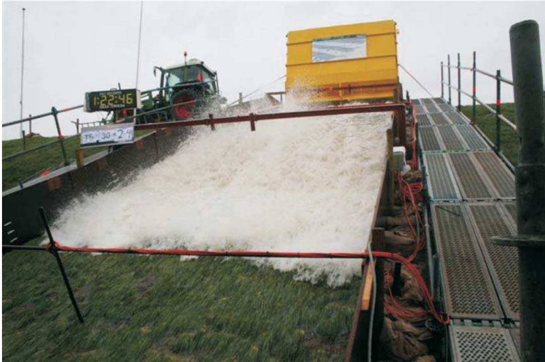
Fig. 3.5: The wave overtopping simulator discharging a large overtopping volume on the inner slope of a dike
