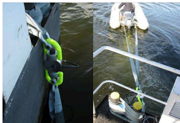
Figure 9 Bollard test, left: used dynamometer, right: test procedure with inflatable dinghy “Avon R340”
