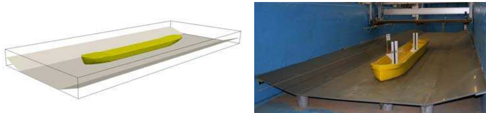
Figure 8. Geometry of the numerical model and the laboratory model
