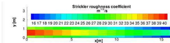
Figure 6. 48 roughness coefficient zones for optimisation problem.
