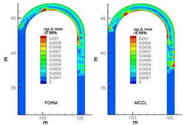
Figure 4. Comparison of the 68 % deviation of bottom evolution according to the friction coefficient calculated with FORM and AD (left) and MCCL (right).
