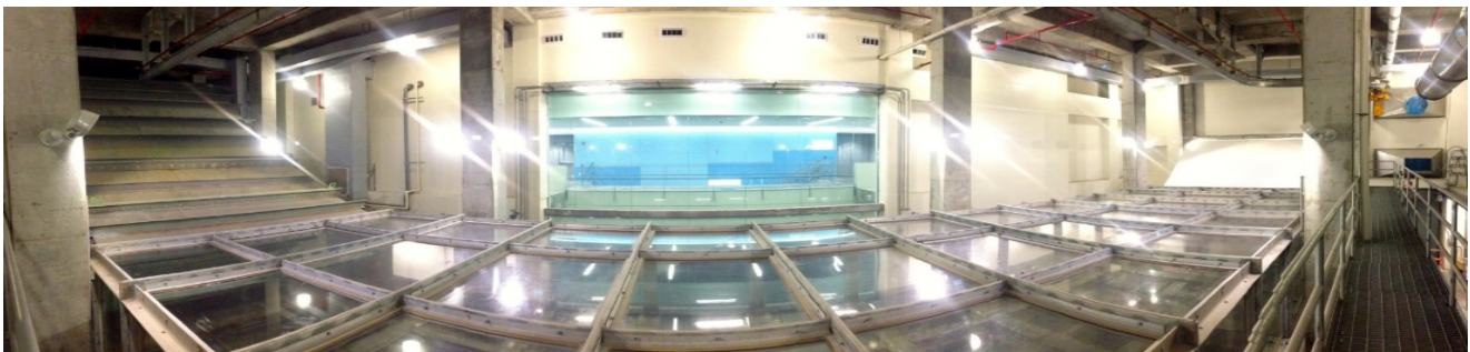
Fig. 1. Panoramic photo of the SUSTAIN tank which has dimensions 21m.-L \times 6m.-W \times 2m.- H.
